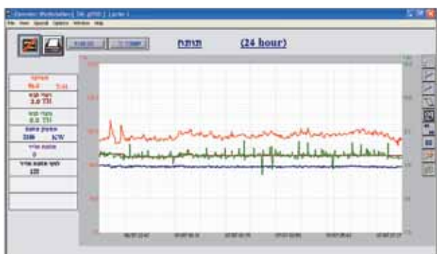
Figure 3. Neshor control panel showing a typical shift after the Silo-Flow™ installation. The green line shows the continuous gypsum feed, closely following the required quantity (brown line) of 3 tph. The red line is the cement production, with an output of around 96 tph.
